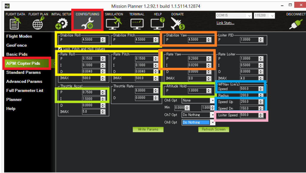
Figure 47: PID Tuning Page in Mission Planner [112]
